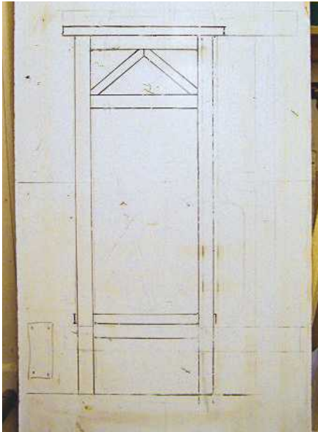
▲ Pic.1 Draw the table out full size on a sheet of faced hardboard to produce a rod to aid the setting out of joints
